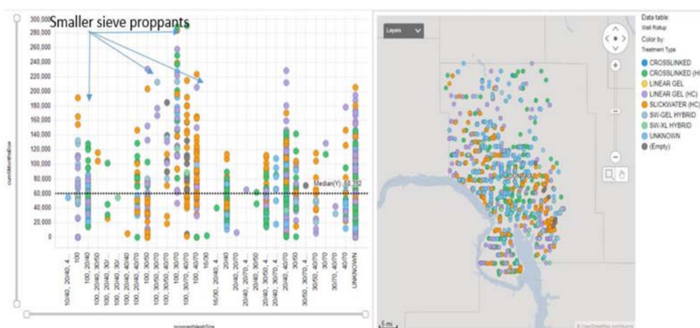
Figure 6—Cumulative 6 mo. Production vs. Proppant Size and Completion Type (Mountrail County 2012 - Present)
